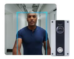
Using  $ACM^TM$  and  $ACC^TM$  software, you can instantly verify if a person seen carding in on camera matches the ID photo associated with the access card they're using, then lock or unlock the door right from your ACC dashboard.
